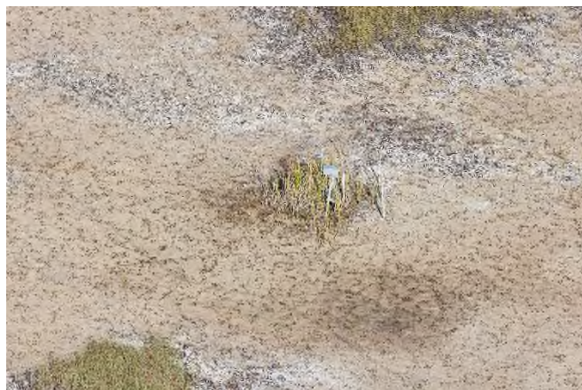
Figure 9. Stage gage registering deeper water than reality.
